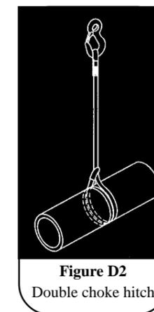
When a sling is used in choke hitch, it should be positioned so as to allow the natural (120°) angle to form and avoid heat being generated by friction. A sling should never be forced into position nor an attempt made to tighten the bite. The correct method of securing a load in a double choke hitch is illustrated in figure D2. A double choke hitch provides greater security and helps to prevent the load sliding through the sling.
