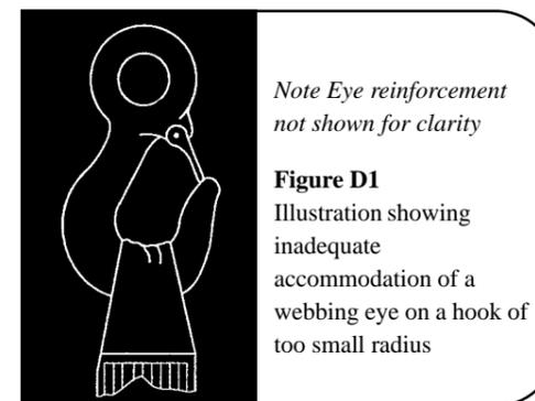
Wide webbing's may be affected by the radius of the inside of the hook as a result of the curvature of the hook preventing uniform loading across the width of the webbing.
